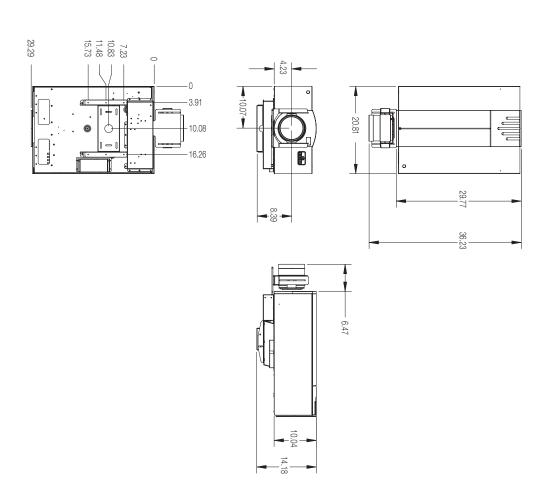
Figure 7-1. VX-33d Dimensions (with Ceiling Mount and CineWide/AutoScope Options)
